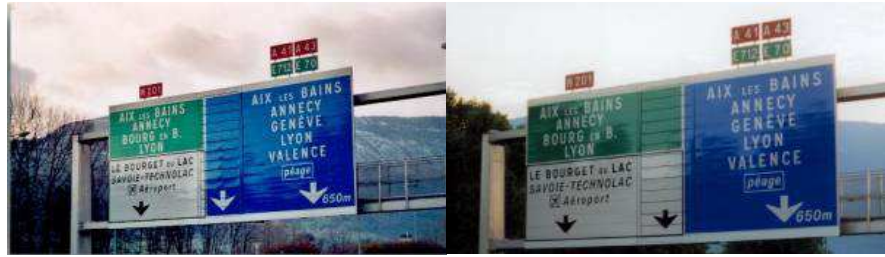
Figure 2.6: An example of destination specific dynamic lane assignment Urban expressway at Chambéry, France (From: Desnouailles et al., 2007)
