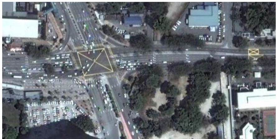
..... Figure 5.28 – Conflict areas indicated by a yellow cross. Stopping in these areas is not allowed.
