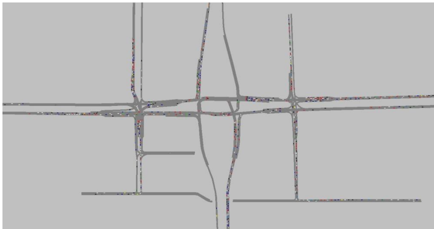
Figure 5.27 – Queues present at all entry links during peak hour traffic simulation (fixed time control)
