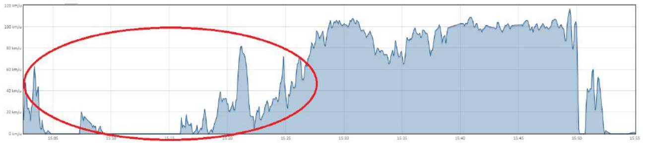
Figure A.22 – Speed profile of a participant's test drive in which congestion is clearly visible
