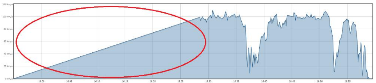
Figure A.23 – Speed profile of a participant's test drive in which congestion is also clearly visible
