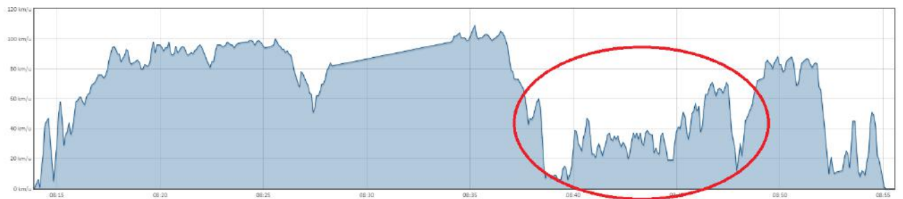
Figure A.22 – Speed profile of a participant's test drive in which congestion is clearly visible
