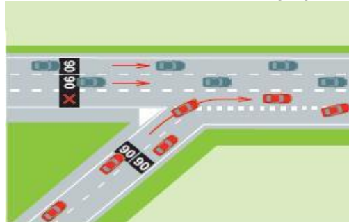
..... Figure B.5: Illustration of Junction Lane Control
